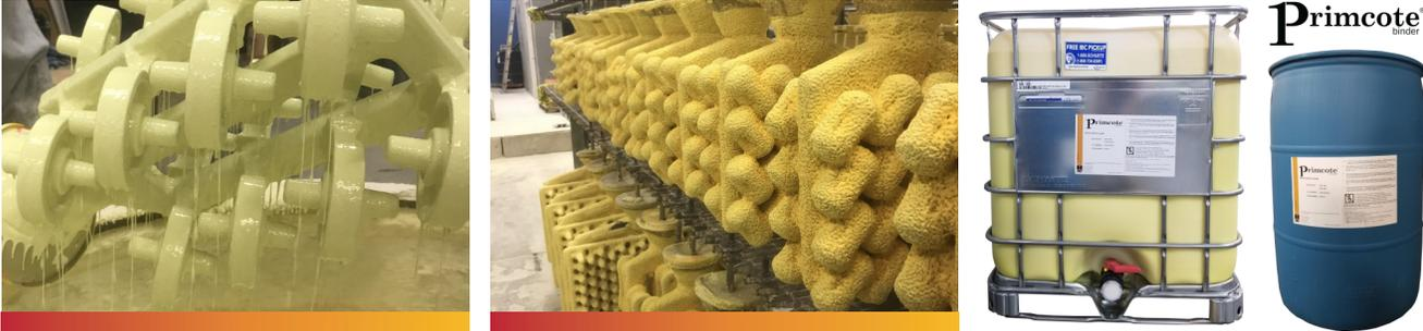
Primcote binder allows faster drying of primary coats with lower humidity and/or increased air circulation. Shell coats using Primcote binder can not be over dried as shell coats using standard colloidal silica can.
