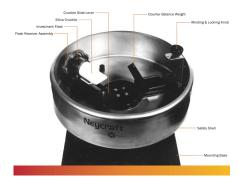
Used to melt and cast metal into the replica investment cavity by centrifugal force, the patented Neycraft centrifugal casting machine is designed with a number of unique operating features.
