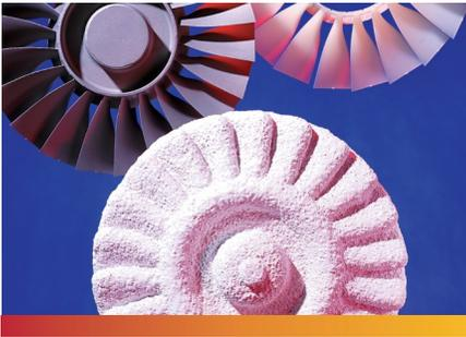
Customcote binder produces strong ceramic shells with many potential benefits over standard colloidal silica and ethyl silicate shells.
