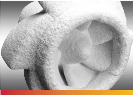
The thinner, yet stronger, shell results in reduced shell material consumption and less shell material for disposal. Shell weights versus standard colloidal silica shells can be reduced significantly depending on the number of shell coats the foundry currently uses.
