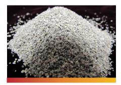
Aluminosilicate is produced from a naturally occurring mineral, calcined mullite, that is precisely sized as either flour or grain. It is available in three alumina contents: 47%, 60% and 70%. The standard alumina content in the investment casting industry is 47%; which provides a very economical and consistent product. These products are low in iron, alkaline and alkaline earth elements.
